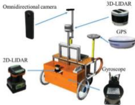
Figure 32. 2017 Hosei University vehicle sensor layout. 13
